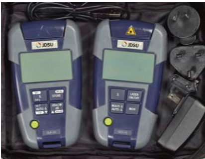
OMK-3x kit with light source, power meter, power supply and USB cable.
